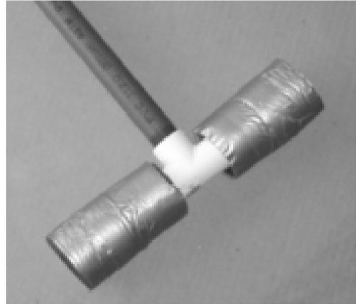
Slide pipe insulation over 3" nipples to cushion mallet head. Use Duct Tape to fasten in place.
